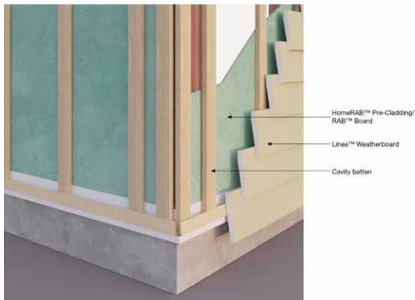
Figure 1: James Hardie Rigid Air Barriers with Linea™ Weatherboard
